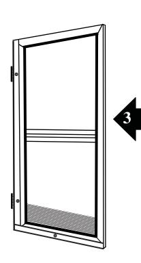
5. Pull the hinge pins and remove door. Slip bottom adjustment channel *over* the hinge channel and bottom door frame. With a hacksaw cut bottom channel even with the width of the door (Fig. 4). Smooth cut edge with a file and return door to the opening.
