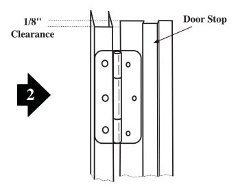
2. Locate position of hinges on door frame while allowing 1/8" clearance at top of hinge channel. Mount hinges with wood screws provided.
