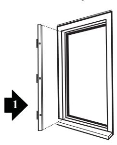
1. Measure height of opening on side where hinges will be fastened (normally same side as the hinges on main door). Cut the bottom of the hinge channel to this measured length, less 2-3/16". File all rough edges smooth. DO NOT cut hinge channel and disregard use of bottom channel if door opening height measures up to ½" over net screen door size.
