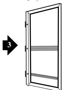
3. Slip the screen door into the hinge channel. With pieces of cardboard, shim door for 3/16" clearance on latch side and 1/8" on top. On outside of door with 1/8" bit drill 2 holes through hinge channel as per illustration. (DO NOT drill completely through door) Follow this same procedure on inside of door and also drilling a third hole at the same height as the push-bar. Insert sheet metal screws provided.
