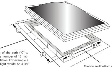
The pitch or down-slope side of the curb ("C" to "D" dimension) determines the number of 12 inch step flashing needed for installation. For example a Tru-Frame® LC2448 model skylight would be a 48" pitch down-slope and would require 8 steps per installation.
