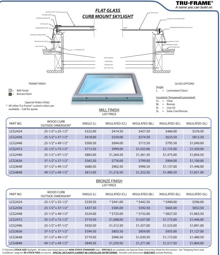
Glass skylights can NOT be manufactured with more than 16 sq. ft. of continuous glass surface. Contact factory for special units. Building Codes vary greatly between States and Counties, and R. Lang Company cannot be held liable for knowing a customer's specific regulations or product application. It is up to the builder/contractor/architect to verify products are within compliance before order is placed.
